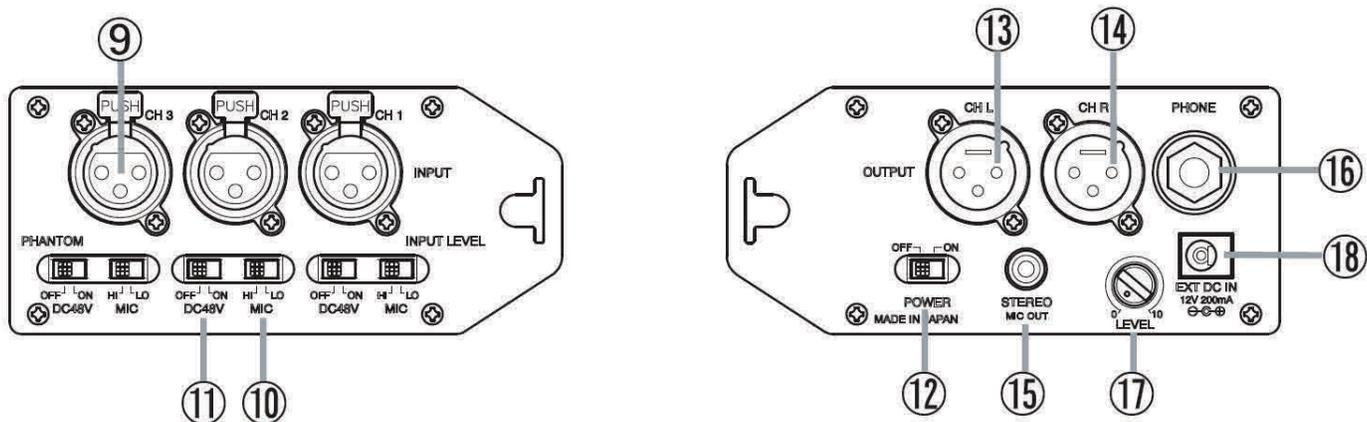
⑨ **CHANNEL 1, 2 & 3 XLR INPUTS:** Connect the 3-pin XLR output of a microphone, wireless receiver or line level audio component to CH 1 and/or CH 2 and/or CH 3. Push the XLR connector into the input jack until it locks. To remove the XLR connector, press the “PUSH” tab while pulling the connector out.
