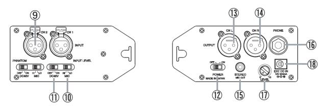
③ CHANNEL 1 & 2 XLR INPUTS: Connect the 3-pin XLR output of a microphone, wireless receiver or line level audio component to CH 1 and/or CH 2. Push the XLR connector into the input jack until it locks. To remove the XLR connector, press the "PUSH" tab while pulling the connector out.
