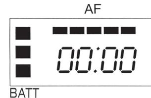
The LCD segments on the left show the approximate remaining battery
