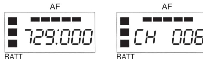
Using either the UP or DOWN button [⑥] the desired receiving frequency or channel number can be set. Tapping the button steps the frequency or channel number one at a time while pressing and holding the button in moves through the frequencies or channel numbers rapidly. There are 121 different frequencies or channel numbers to choose from. Once the desired frequency or channel has been determined be certain to set both the transmitter and receiver to match.
