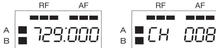
Using either the UP or DOWN button [⑩] the desired receiving frequency or channel number can be set. Tapping the button steps the frequency or channel number one at a time while pressing and holding the button in moves through the frequencies or channel numbers rapidly. There are 121 different frequencies or channel numbers to choose from. Once the desired frequency or channel has been determined be certain to set both the transmitter and receiver to match.
