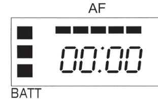
The LCD segments on the left show the approximate remaining battery life (from 1 to 3 segments) with 3 segments meaning maximum battery power. The bottom segment will blink when the battery power falls to less than 6.2V and indicates that it is time to replace the battery. Azden recommends the use of Alkaline batteries only.
