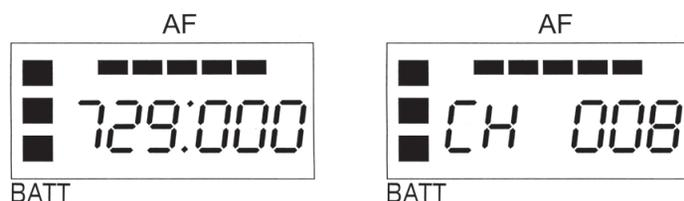
Using either the UP or DOWN button [⑩] the desired receiving frequency or channel number can be set. Tapping the button steps the frequency or channel number one at a time while pressing and holding the button moves through the frequencies or channel numbers rapidly. There are 121 different frequencies or channel numbers to choose from. Once the desired frequency or channel has been determined be certain to set both the transmitter and receiver to match.
